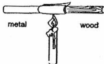
The joint was heated by a candle flame for a few seconds. It was observed that the part of paper around the metal rod showed no change while the part of paper around the wooden rod was slightly burnt.
