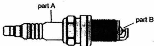
Part A of the spark plug in contact with the combustion chamber has to be insulated from extremely high temperature. Part B of the spark plug is a conductor of electricity for spark production.
