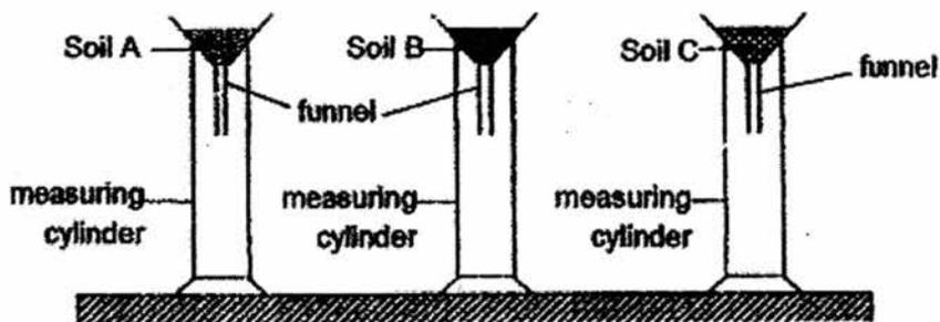
She then poured 150 ml of water into each funnel and measured the time taken to collect 50 ml of water in each of the measuring cylinder. The graph below shows the results of her experiment.
