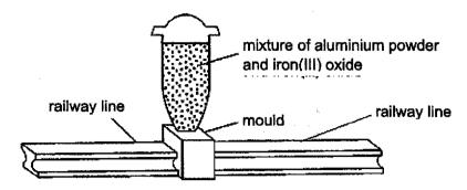
The mixture is ignited and an exothermic reaction takes place. The molten iron formed is collected in the mould. The molten iron solidifies and repairs the crack between the rails. The mould is then removed.
