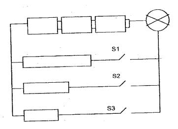
Kelvin closed switch S1 and kept switches S2 and S3 open. He then observed the brightness of the bulb. He repeated the experiment by closing switch S2 and keeping switches S1 and S3 open. Once again, he observed the brightness of the bulb. He did the same with switch S3. At any time, only one switch was closed.
