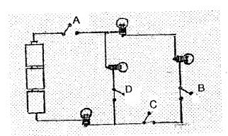
When all the switches are closed, all the bulbs light up. Jamie wants to open one switch which will switch off all the bulbs. Which switch should she open?
